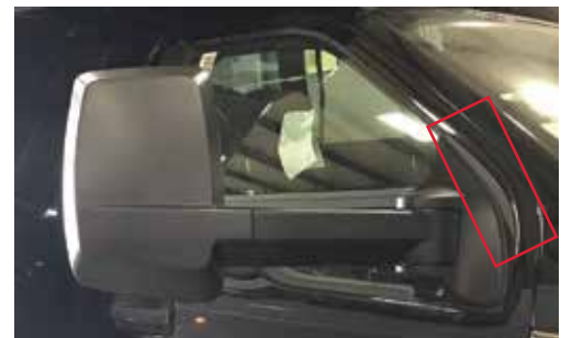
Adapter kit installed on mounting base of F550.
