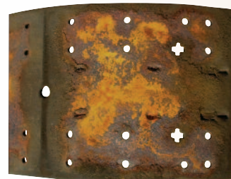
The strength of Marathon's linings make them better able to withstand the effects of rust jacking on a brake shoe.
