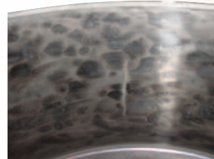
Brake drum showing damage from competitor's material
