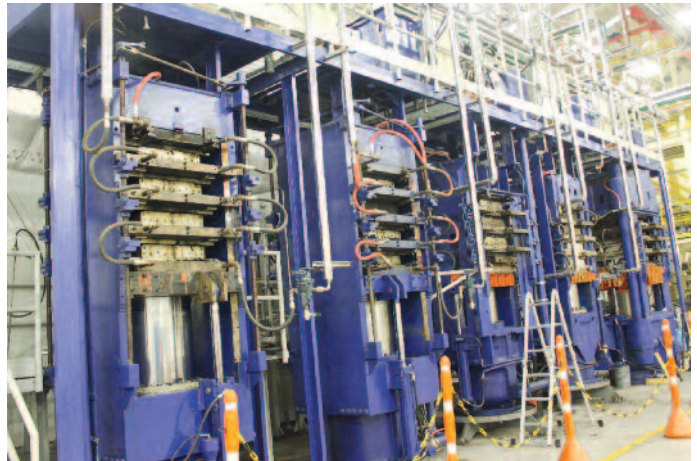
Computer controlled hot presses ensure optimal product curing
