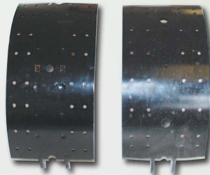
Marathon Brake shoes after 24-hours of salt-spray exposure.
