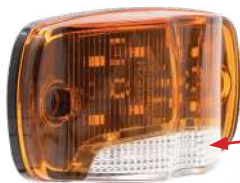
DOWNWARD GROUND ILLUMINATION LIGHT
