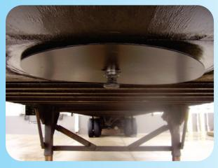
The steel ring was always the "weak link" in previous designs and often was not secure enough to keep the disk in place. As a result a damaged ring could prevent a successful lock between king pin and 5th wheel.
