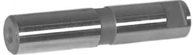
Spring Pin; 1" O.D. x 4 13/16" Lg. x 1/2" CE; Front
