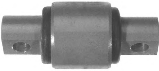
Bushing; 2 17/32" O.D. x 4 3/8" C to C; Model EF/ER w/ 3" Wide Springs
