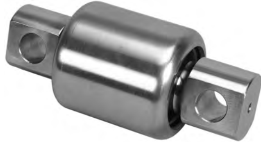
Bushing, Urethane; 2 3/4" O.D. x 4 3/8" C to C, 5/8" Bolts, 1 1/4" Rod; Model SS34/38/ST34
