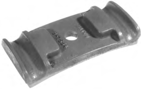
Saddle, U-Bolt; 10 7/8" Lg. x 5" W, 8 5/8" C to C; Model SS58/65/SWS59
