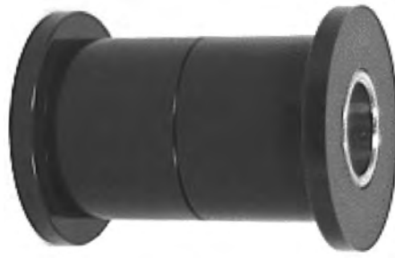
Bushing, Urethane; 7/8"ID x 1 29/32"OD x 3"Lg.
