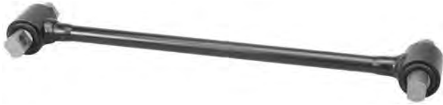
Track Rod, Rigid; 23 15/16"Lg; Solid Spacer; Model FASII Airliner (1990+)
