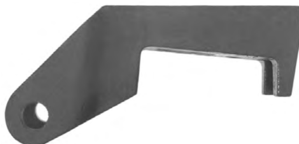
Bracket, Torque Rod Seat; Casting #47982, 47962; 8.00° Pinion Angle; Model E4 360/400
