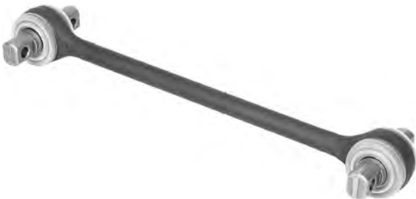
Torque Rod, Rigid; 22 1/4"; Full ball ends; Model VOAS Corporate Air Suspensions
