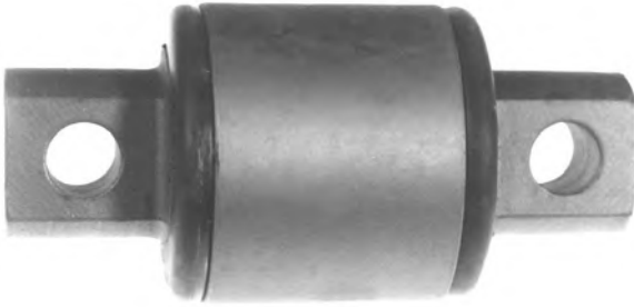
Bushing; 2 3/4" O.D. x 4 3/8" C to C, 5/8" Bolts, 1 1/4" Rod; Model SS34/38/ST34
