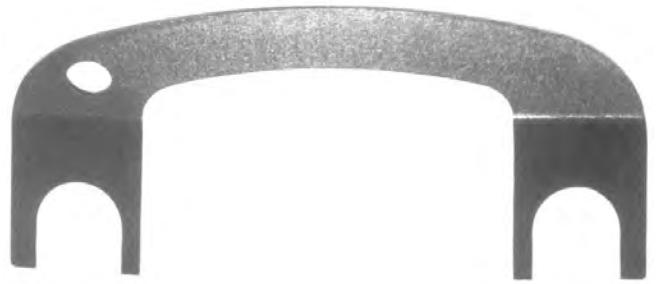
Shim; 1/16" Thk.; 4 3/8" C to C; Models Corporate Air Ride, Four Spring
