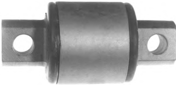
Bushing, Straddlemount; 2 3/4"OD x 4 3/8" c/c; For 5/8" Bolts and 1 1/4" Forged Rod; Models Glide Ride, Airglide 100, "Big 6"
