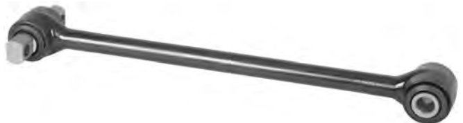
Torque Rod; 22 1/4" Lg; 7/8" ID; Straddle Mount End; Model Maxlite 40EZ
