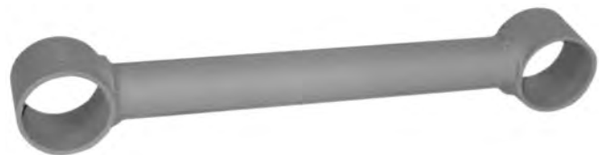
Torque Rod, Rigid; 21 1/2" Lg.; Type O and I Joints; Use w/ 321-273 Bushings; Models 600/800 Truck Suspensions, 700 Trailer Suspension
