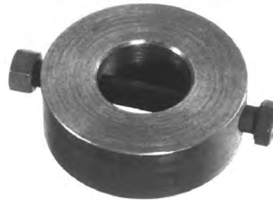
Collar Assembly; 1 1/4" I.D. x 2 3/4" O.D. x 15/16" Thk.; 3/8"-16 x 3 1/4" Lg. Bolt; Model 1400
