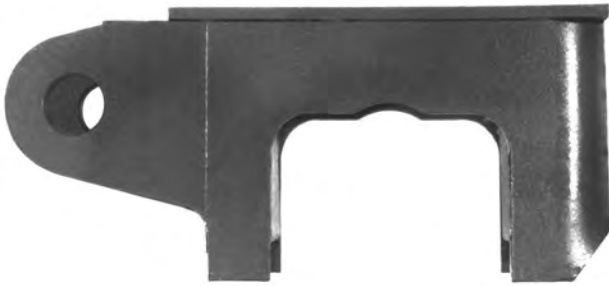
Bracket, Torque Rod/Seat; HEIGHT = 1 3/4"; 4" x 6" Axles; Use w/ 334-344 T/R Bolt and Bushing Assy.; Model "Standard"
