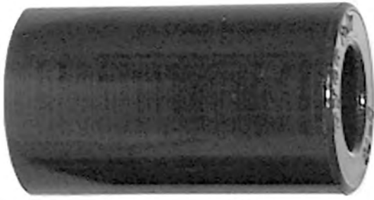
Bushing, Urethane; 7/8"ID x 1 1/2"OD x 2 3/4"Lg.
