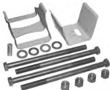
Service Kit, Clamp Group; 8 1/2" ride height; incl 334-1731 <10/12; Models Airtek/Softek
