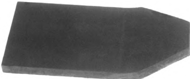
Plate, Beam End Repair - All Beams; Replace Beam When Beam Wear Exceeds .030"; Models 600/800 Truck Suspensions, 300/700 Trailer Suspensions
