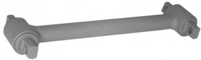
Torque Rod, Rigid; 18 1/8", 1 15/16" O.D. Tube; Includes 321-279 Bushings; Model Corporate Four Spring, Corporate Air
