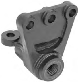
Hanger, Shackle; LH/RH; 2 1/4" from Bottom of Frame to C/L 3 Holes; TB-78; 11 13/16" frame; Models VN, Mack CXN
