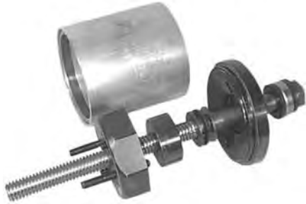
Tool, Bushing Installation; Tri-Functional® Bushings; Model Toughlift
