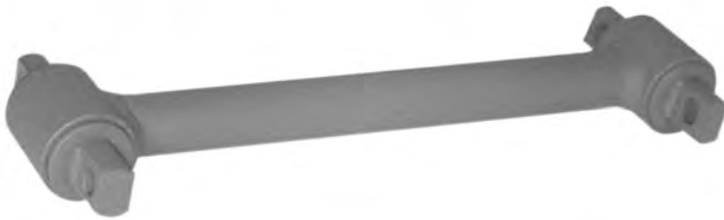
Torque Rod, Rigid; 18 1/8" C to C Tubular, 1 9/16" O.D. Tube; Includes 321-323 Bushings; Model Corporate Four Spring, Corporate Air
