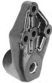
Hanger, Shackle; Incl. 321-141 bushing; Models Columbia, Coranado, Cascadia, Argosy, Condor
