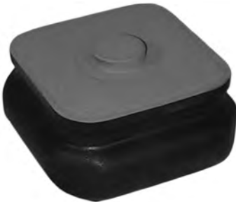
Insulator, Urethane Extra Service; 3 3/4" Thk. x 6" W x 6" Lg.; 1 3/4" Dowel; 80 Durometer, Urethane
