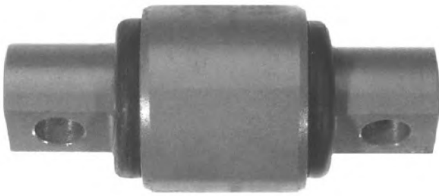
Bushing; 2 17/32" O.D. x 4 3/8" C to C; 5/8" Bolts; Models Corporate Air Ride, Rear Single Axle, Four Spring
