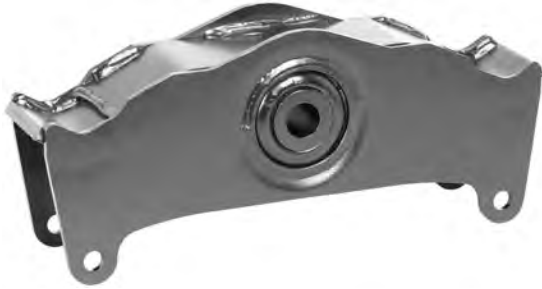
Equalizer Assembly, Fabricated; 17 3/8" OAL; 321-221 Bushing; 50" Axle Spacing; Replaces 338-1536; Models 9600, 9700
