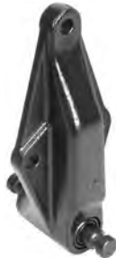
Hanger, Shackle; Incl. RB-249 bushing; Front
