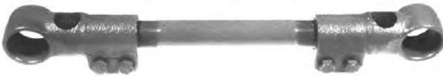
Torque Rod, Adjustable; 18"-20" Lg.; Use w/ 321-177 Bushings, 334-640 T/R Bolt and Bushing Assy.; Model H
