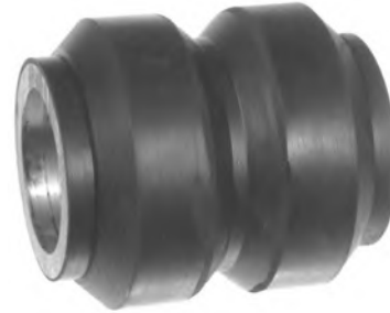
Bushing; 2" I.D. x 3 1/2" O.D. x 4" Lg.; Included in 334-819 Bolt and Bushing Assy.; Model NF-2
