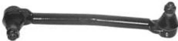
Ball stud dimensions different on both ends
