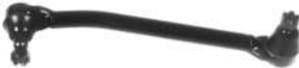
Ball stud dimensions different on both ends
