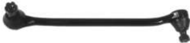
Ball stud dimensions different on both ends
