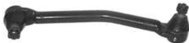
Ball stud dimensions different on both ends
