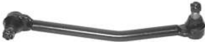
Ball stud dimensions different on both ends
