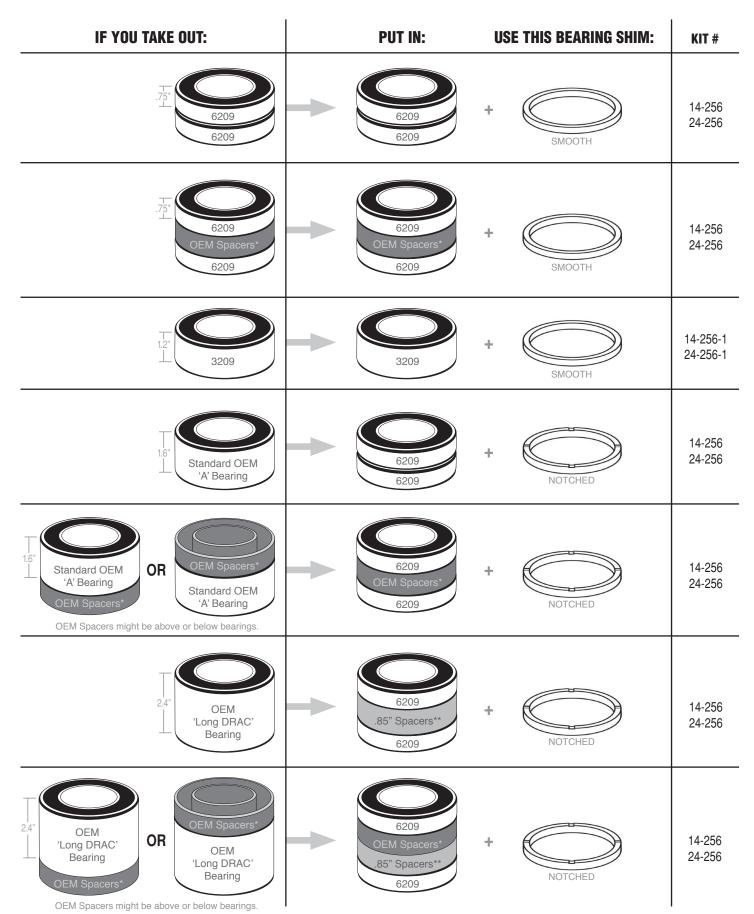
\*OEM Spacers heights vary. Always reuse any and all bearing spacers from OEM fan clutch. Bearing spacers always come in pairs - an inner and outer race. Failure to use both spacers will cause bearing failure
