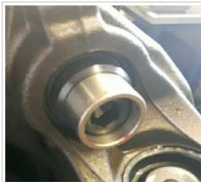
This Rubber/ Metal Bush is the old design revision that Knorr-Bremse replaced some time ago. Fraser Gauge upgrades the most recent.
