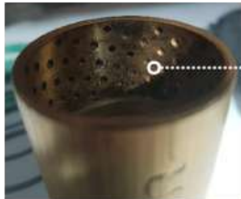
Evidence of previous use and score marks present where an attempt has been made to polish away.
