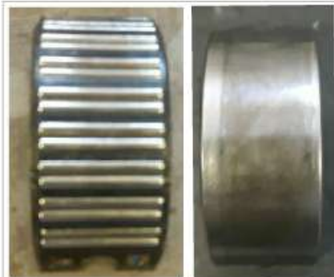
The Needle Rollers & Shells had been re-used. The Needle Rollers especially are a wearing part.
