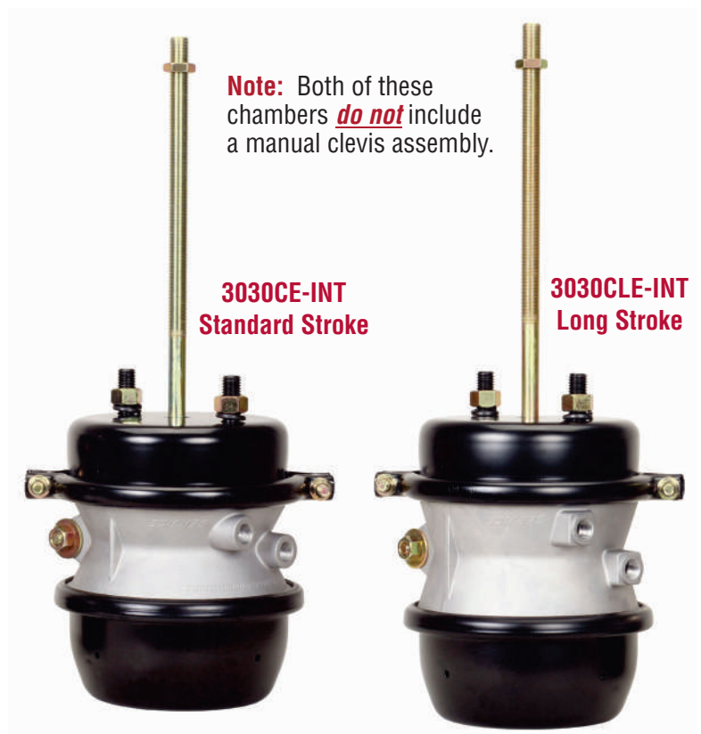
The 3030CLE-INT long stroke has square shaped ports to identify it is a long stroke air chamber.
