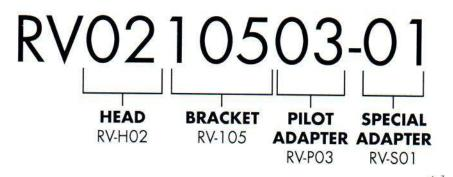
The first two components (head and bracket) are always required, but not all clutches contain a pilot adapter or special adapter. If one of these components is not required, there will be double zeros. So for example RVO210500-01 would mean that there is not a pilot adapter, since there are double zeros in the pilot adapter section of the part number, but there is a special adapter (RV-S01)
