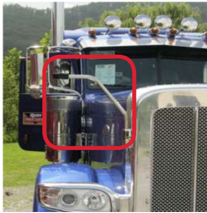
1" OD stainless steel tubing arm can be rotated for fine camera angle adjustment. Also rotates upon impact to reduce the potential damage
